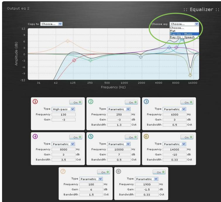
Figure 7: Set the equalization for Ray-On columns in the output equalizers
