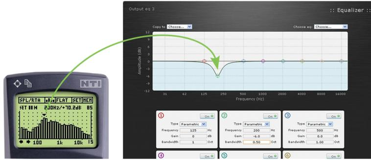
Figure 11: Equalize loudspeakers -> microphones feedback in the output equalizers
