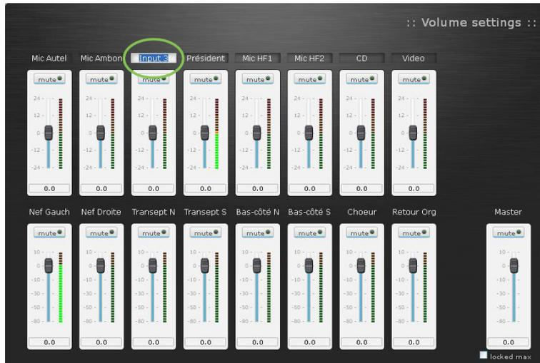
Figure 3: Name the inputs and outputs in the Volume block-function
