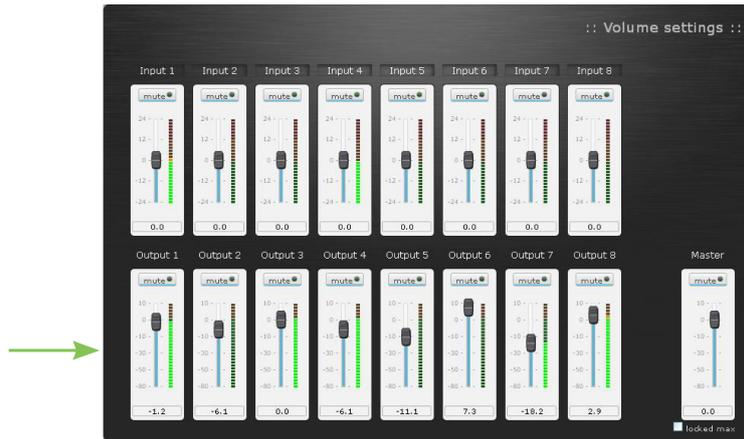
Figure 9: Adjust the sound coverage with the output gains in the Volume block-function
