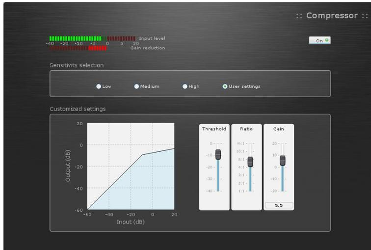
Figure 5: Compressor block-function interface
